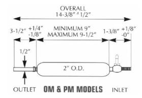
All OM models supplied with 1/2" OD smooth tube connection unless otherwise specified. OM<sup>-3</sup> Range leaks provided with 500-cc volume.
