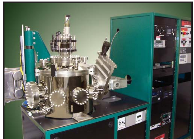
ATC 2200 IBAD with (3) A340-XP 4" UHV sputter sources with in-situ tilt, a COPRA ICP plasma/ion source for ion beam assisted deposition below 5 \times 10^{-4} Torr, 1200 l/s turbopump, 800°C rotating substrate heater with RF bias, computer control and a load-lock for 6" diameter substrates.
