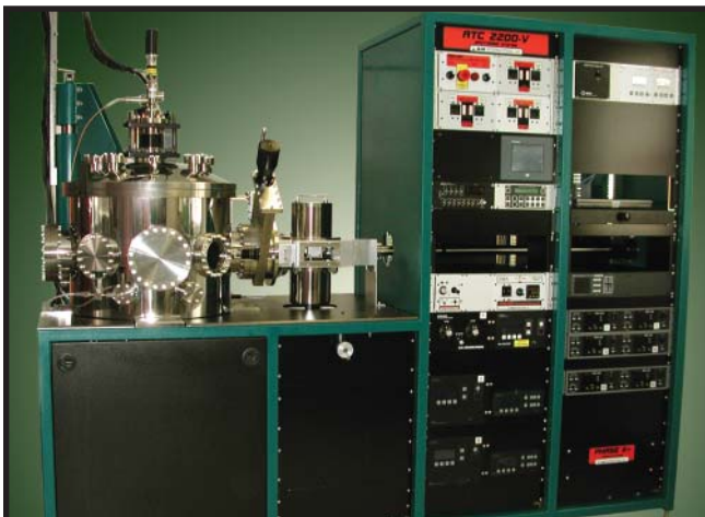
ATC 2000 with (6) A320-XP 2" UHV sputter sources with in-situ tilt, 1200 l/s turbopump, 850°C rotating substrate heater with RF bias, computer control and (6) substrate cassette elevator in the load-lock for 4" substrates.
